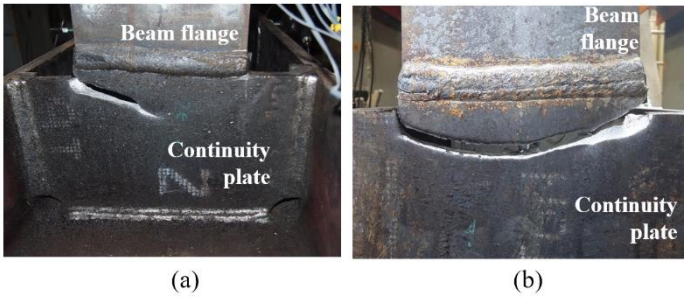
Fig. 5. Fracture in the continuity plates of Specimens: a) W1, and b) W2
