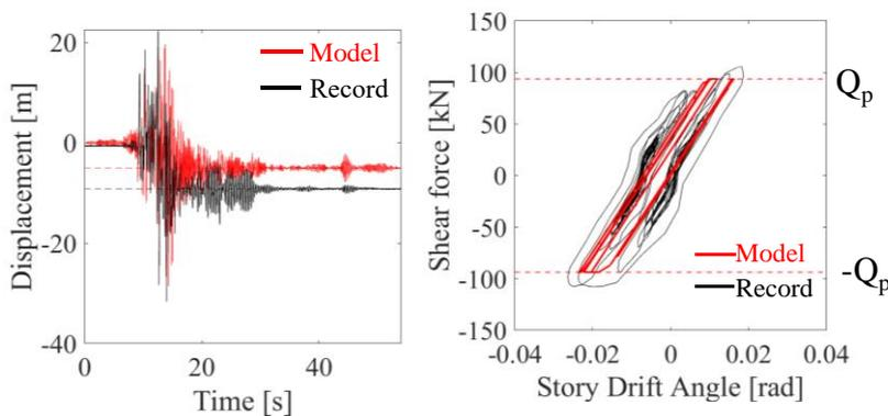
Fig. 16 Result of elastic-plastic analysis of single degree of freedom: (a) Displacement response, (b) Shear force and story drift angle relationship
