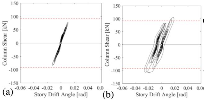
Fig. 9 Shear force and story drift angle relationship: (a) test 3, (b) test 5.
