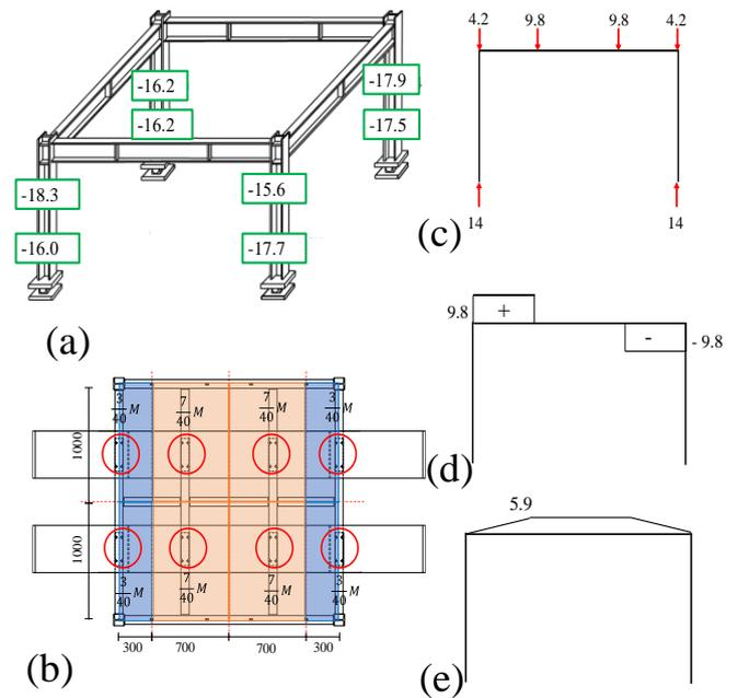
Fig. 5 Initial condition and assumptions before excitation: (a) Measured axial force of column, (b) Assumed mass distribution, (c) Assumed concentrate load, (d) Assumed shear force diagram
