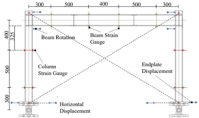
Fig. 4 Instrumentation plan
