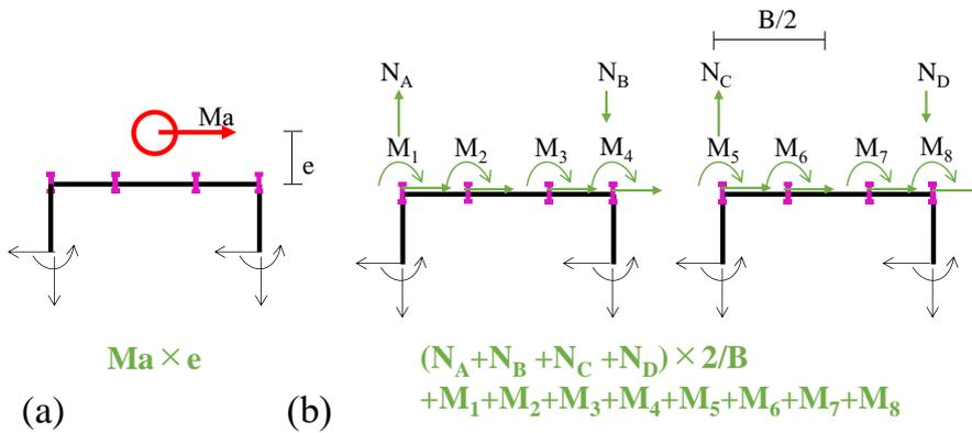
Fig. 13 Expected moment by ground motion: (a) Inertial force (b) Transferred force
