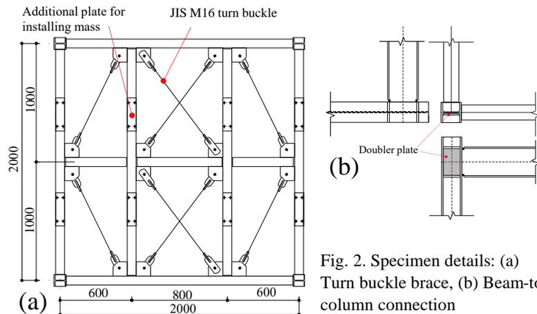
Fig. 2. Specimen details: (a) Turn buckle brace, (b) Beam-to-column connection
