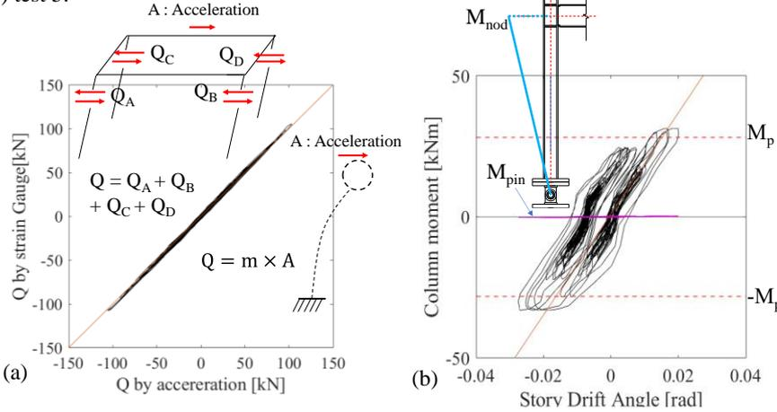
Fig. 12 Verification of forces: (a) Shear force by column shear and condensation models, (b) Relationship of column top moment and pin moment
