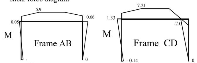
Fig. 6 Initial bending moment diagram combine assumption with measured axial force: (a) Frame AB, (b)
