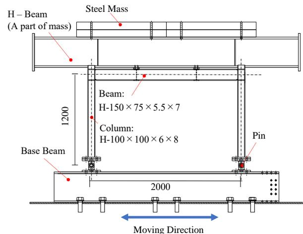
Fig. 1. Test specimen
