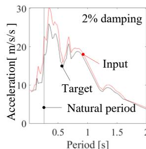
Fig. 7 Record of absolute acceleration response
