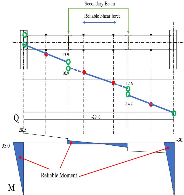
Fig. 14 Calculation method of torsional moment of secondary beam
