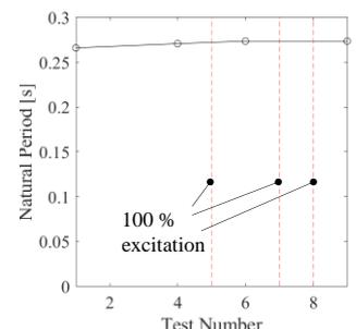
Fig. 8 The change in fundamental vibration period
